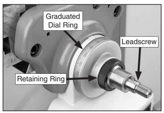
Figure 59. Power feed ball handle removed.
